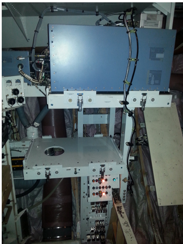
Figure 4. Picture of the IAGOS system setup in the avionics bay. The pump box (small blue box in the upper left corner) embeds the pressurization pumps that drive the outside air collected through the pitot (see Fig. 3c) to Package1 (P1; big blue box). The system functioning and safety are managed via the control panel and relay panel seen in the lower part of the picture. The empty shelf is available for Package2 instruments also developed within the IAGOS program.
