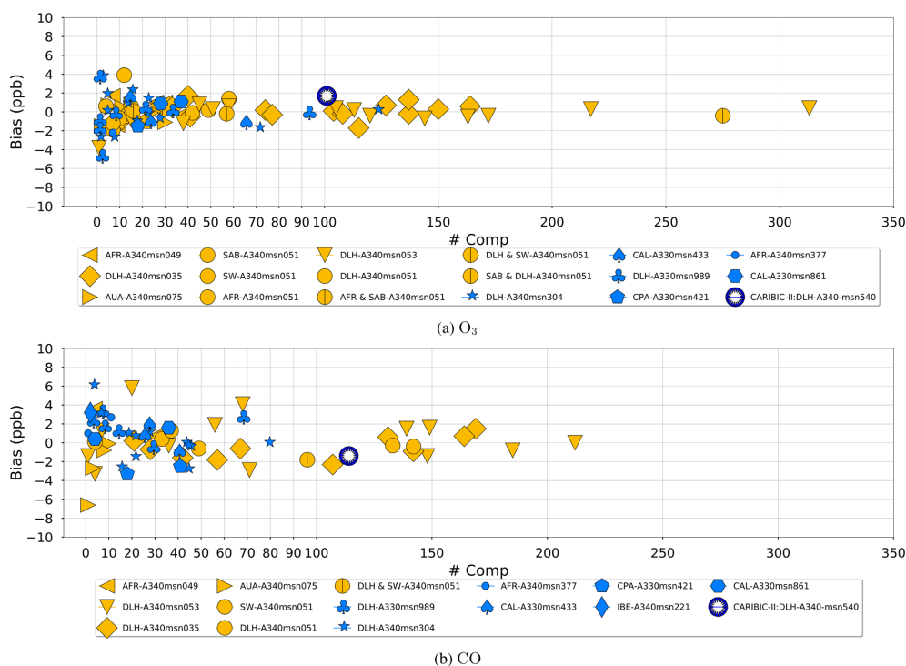
Figure 11. Dependency of the O 3 (a) and CO (b) instrument measurement mean bias for each FP with the number of flight intercomparison profiles. Different symbols are used for each distinct aircraft (same as Fig. 10); the yellow color is for the MOZAIC program and the blue color is for IAGOS and CARIBIC.
