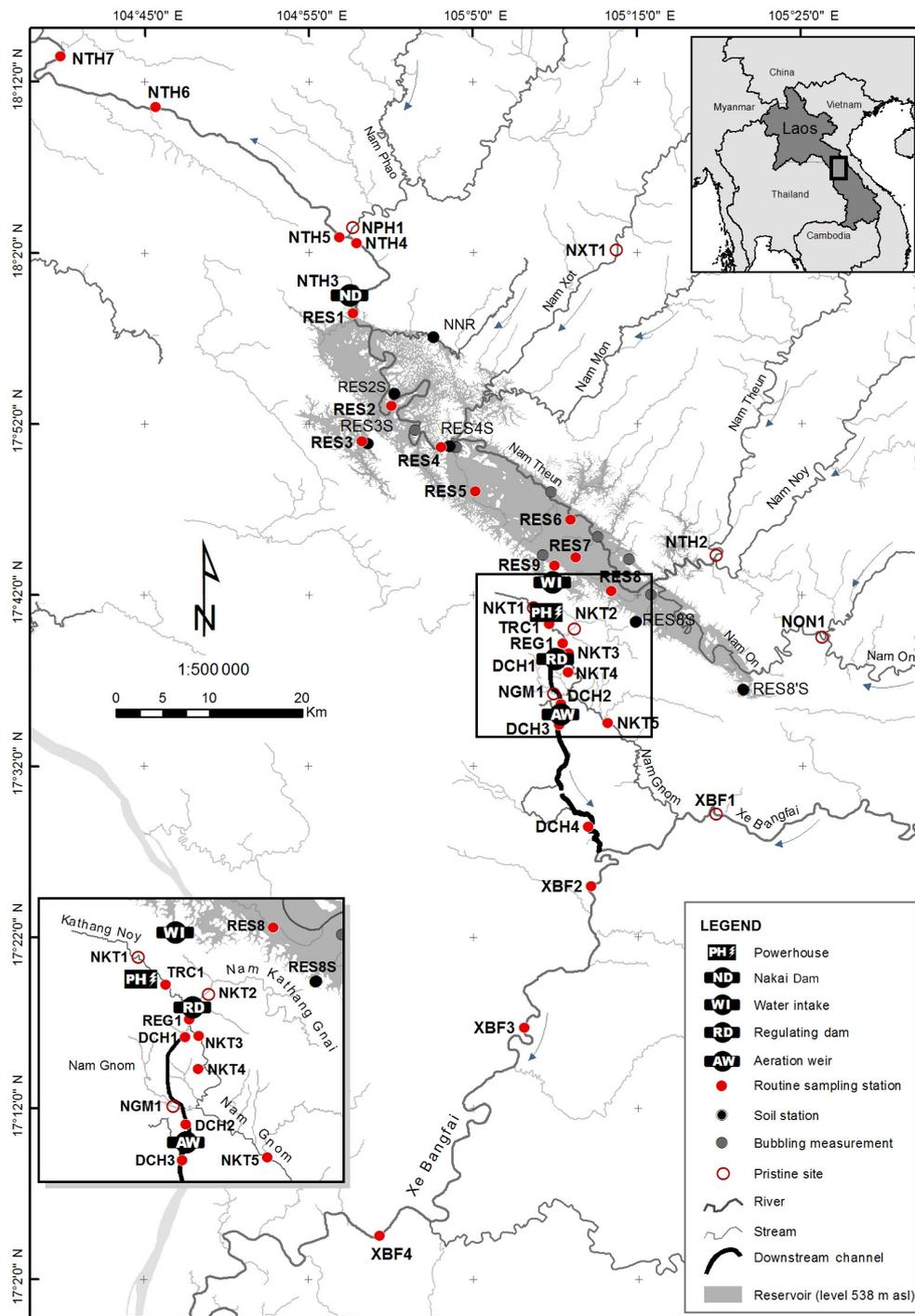
**Figure 1.** Map of the Nam Theun 2 monitoring network. The station names are defined by numbers and an abbreviated name as follow: RES standing for reservoir, NTH for Nam Theun River, NON for Nam On River, NXT for Nam Xot, NPH1 for Nam Phao River, TRC for tail race channel, REG for regulation pond, DCH for downstream channel, NKT for Nam Kathang River, NGM for Nam Gnom and XBF for Xe Bangfai River.
