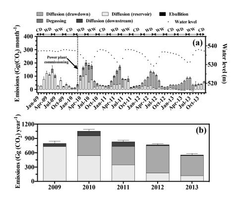
**Figure 8.** Monthly (**a**) and yearly (**b**) average of the total emissions from the Nam Theun 2 Reservoir by diffusion at the reservoir surface, diffusion from the drawdown area, ebullition, degassing and diffusion from the Nam Theun River and artificial channel at the Nam Theun 2 Reservoir (Lao PDR). In panel (**a**), water-level variations in the reservoir are also given.
