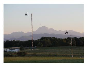
**Figure 1.** The figure is showing the two main measurement towers and the Pyrenees mountain range in the background. The small divergence site tower is marked with A and taller 60 m tower is marked with B.
