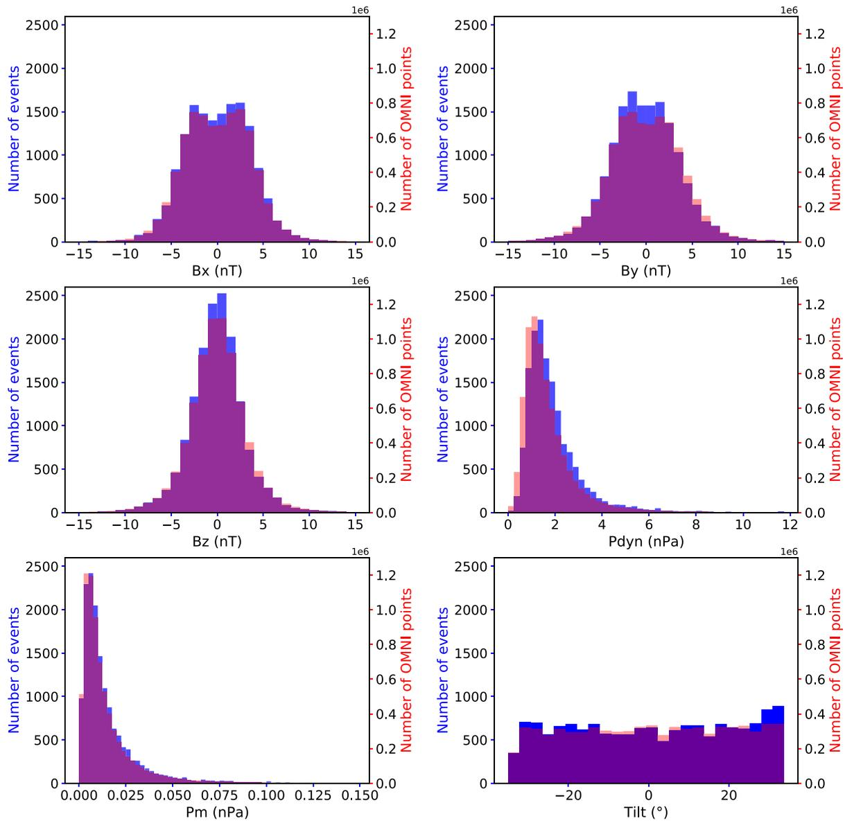
**Figure 1.** Statistical distribution of the solar wind parameters of the 17,230 magnetopause crossings: the three magnetic field components,  $B_x$  (top left),  $B_y$  (top right),  $B_z$  (middle left), the dynamic pressure  $P_{dyn}$  (middle right), the magnetic pressure  $P_m$  (bottom left) and the dipole tilt angle (bottom right). The red bins indicate the counterpart distribution of the physical parameters of OMNI data between 2001 and 2019.
