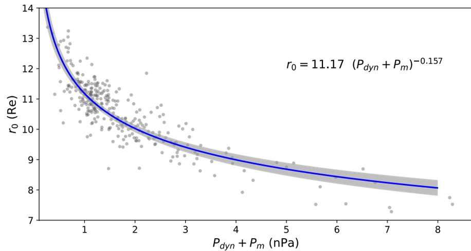
**Figure 4.** Variations of  $r_0$  with the dynamic pressure. The solid blue line represent the fit of  $r_0$  as a power-law of  $P_{dyn} + P_m$  and the gray interval is the 1-sigma confidence interval of such fit.
