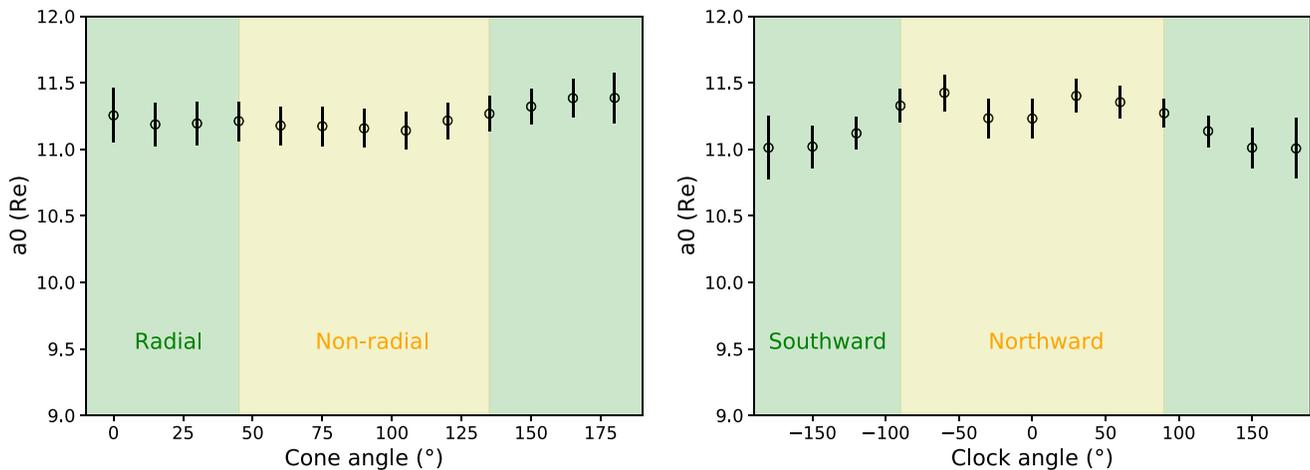
**Figure 5.** Evolution of the stand-off distance at 1 nPa,  $a_0$  as a function of the interplanetary magnetic field cone (*left*) and clock (*right*) angles. The black circles represent the value we obtain from fitting a power law to  $r_0$  for different cone (resp. clock) angle bins. The error bars represent the 1-sigma confidence interval of such fits.
