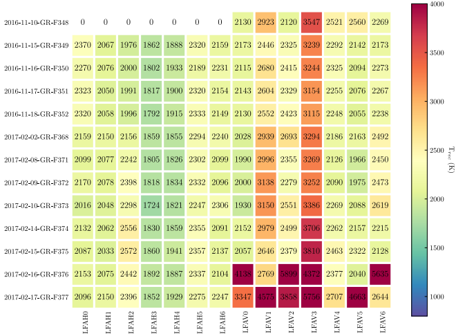
Fig. A.6. Summary of upGREAT LFA single-sideband receiver temperature for the 13 project flights. The receiver temperature for the V array increases toward later flights. This was linked to a degradation in LFAV LO performance. The LO was shipped back to the manufacturer for maintenance after the flight series. The H LO was not available during the 2016-11-10 flight and is recorded here with 0 receiver temperature.
