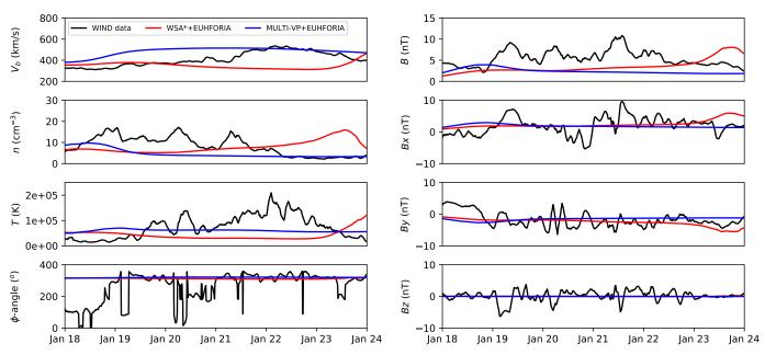
Fig. 10. Plasma and magnetic parameters at 1 AU as modeled by WSA\*+EUHFORIA-heliosphere (red) and MULTI-VP+EUHFORIA-heliosphere (blue) with a WSO magnetogram (CR2199). The observed data as captured by WIND are depicted in black for the HSS that reached Earth on 2018-01-21.
