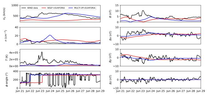
Fig. 12. Plasma and magnetic parameters at 1 AU as modeled by WSA\*+EUHFORIA-heliosphere (red) and MULTI-VP+EUHFORIA-heliosphere (blue) with a GONG magnetogram. The observed data as captured by WIND are depicted in black for the HSS that reached Earth on 2011-06-22.
