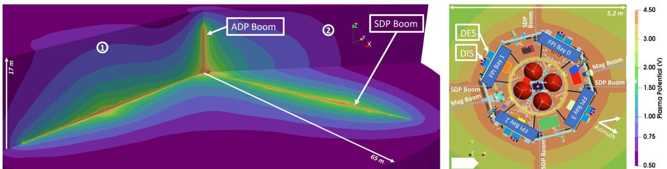
**FIG. 3.** Ambient potential as calculated by the SPIS model. The left panel shows an orthographic cutout. The right panel shows a zoom in of the area near the spacecraft, with the MMS spacecraft overlaid showing instrument locations. Annotations show the boom locations as well as the FPI sensor locations. Note that similar DES/DIS pairs are in all four of the annotated FPI bays. The azimuth angle for all future figures is as annotated here as is the direction of the Sun.
