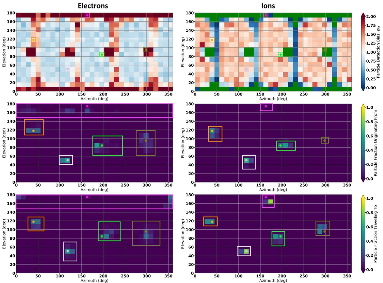
**FIG. 10.** Indications of where, for a given look direction (colored dots), a particle with that look direction at infinity is detected (bottom) and where a particle detected from that look direction originated at infinity (middle), for electrons (left) and ions (right). Colored outlines indicate the approximate area of influence for the matching colored look direction. The bias maps ( $\sim 10\text{--}13$  eV) are the same as in Fig. 4.
