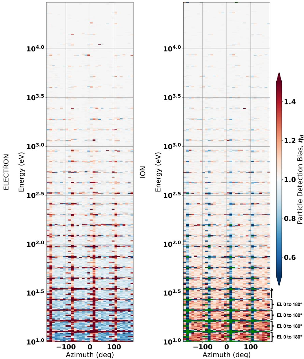
**FIG. 6.** Detection efficiency map corresponding to an FPI energy/angle sky map for electrons (left) and ions (right). Green coloring denotes areas where no detected particles originated in the simulation domain.
