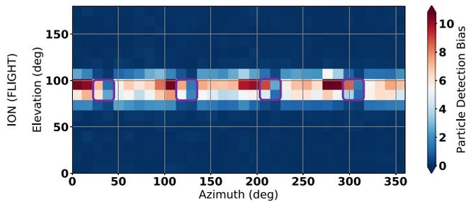
**FIG. 5.** Detection bias map ( $\sim 10$ – $13$  eV) for DIS flight data from MMS3 on December 28, 2016. A narrow ion beam which swept around the spacecraft as it spun was dramatically reduced in intensity when coming from the look direction of the SDP wire booms. Purple squares represent the approximate look direction of the SDP.
