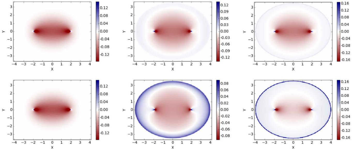
**Figure 8.** Comparison of isotropic (left), anisotropic (centre) and isotropic-equivalent (right) intensity kernels for scattering perturbations (see the text for a definition of ‘isotropic-equivalent’). The top and bottom plots correspond to weak ( $g = 0.5$ ) and moderate ( $g = 0.8$ ) anisotropic scattering, respectively.
