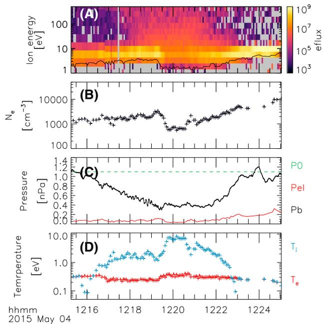
**Figure 2.** Estimates of ion temperature within the heating event. (a) Ion energy; (b) electron density; (c) magnetic pressure (black, calculated from data), electron pressure (red, calculated from data), and total pressure (green dashed line, assumed constant and equal to the sum of the magnetic, electron and ion pressures); (d) electron temperature (red), estimated ion temperature needed to conserve total pressure (blue).
