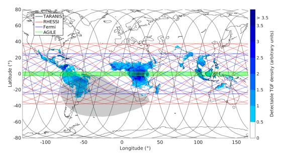
Figure 4. Estimated global detectable TGF density map, and ground tracks of the orbits of TARANIS (planned), RHESSI, Fermi and AGILE. The grey area denotes an approximative South Atlantic anomaly assumed for the simulations, and where TGF can occur but no detection by satellites is possible due to high background.
