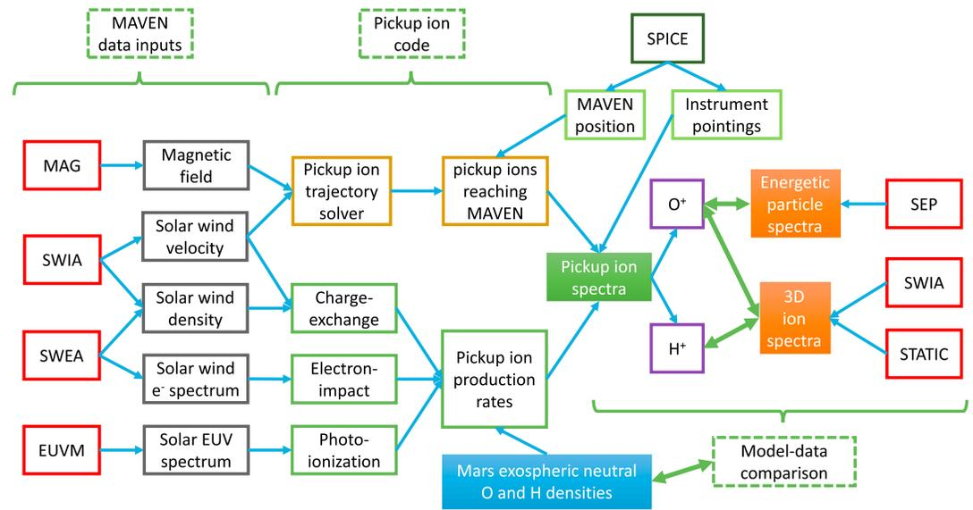
**Figure 1.** Different working parts of the pickup ion code used in this study. Data from the MAVEN MAG, SWIA, SWEA, and EUVM instruments are used in calculating pickup ion spectra seen by the SEP, SWIA, and STATIC instruments. Model-data comparisons help in constraining the Mars exospheric neutral densities and the associated neutral escape rates.
