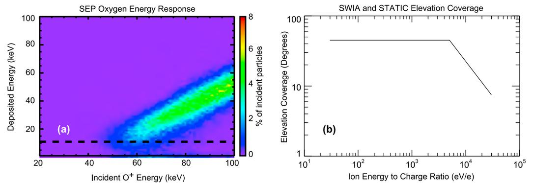
**Figure 3.** (a) Energy response of SEP to incident oxygen ions. SEP's electronic noise threshold is 11 keV and is marked by the dashed line. Oxygen ions with energies above  $\sim 60$  keV trigger counts in SEP. (b) Dependence of the SWIA and STATIC's deflection angle (elevation) coverage on the energy of the measured ions. Below 5 keV, the elevation coverage is  $\pm 45^\circ$ . Above 5 keV, the elevation coverage drops proportional to the energy and reaches  $\pm 7^\circ$  at 30 keV.
