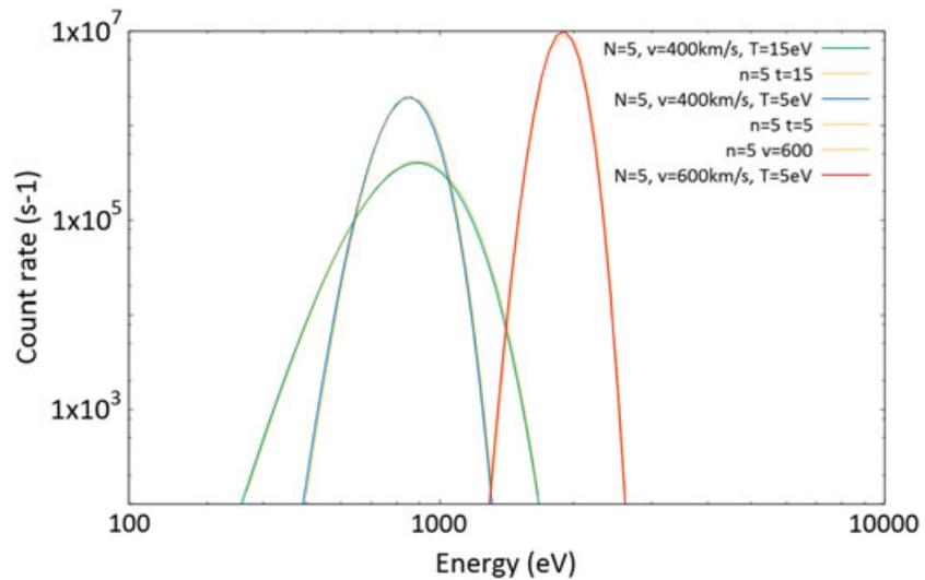
**Figure 11.** Count rate estimated for a 3° azimuthal angular sector in the present design. There are curves for three types of solar wind: typical slow ( $T = 5$  eV and  $V = 400$  km/s) and fast ( $T = 15$  eV and  $V = 600$  km/s) winds, as well as a very unusually hot and slow wind for context ( $T = 15$  eV and  $V = 400$  km/s). For each type of wind, the count rates have been estimated by using both SIMION and Trace simulations.
