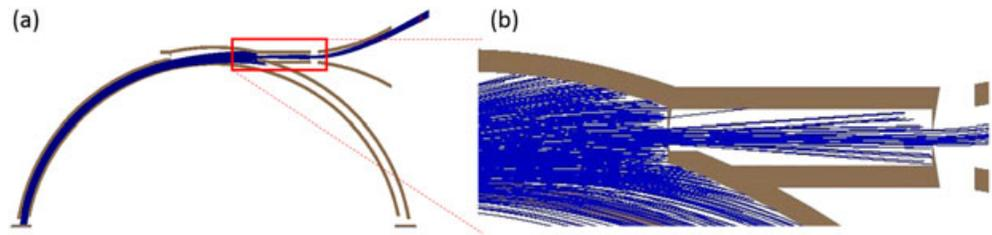
**Figure 5.** (a) Actual design with sample particle tracing (particles are launched from the detectors on the bottom left) and (b) zoom-in on the collimator area to highlight its importance in determining the elevation of accepted particles, and in turn elevation and energy resolutions.
