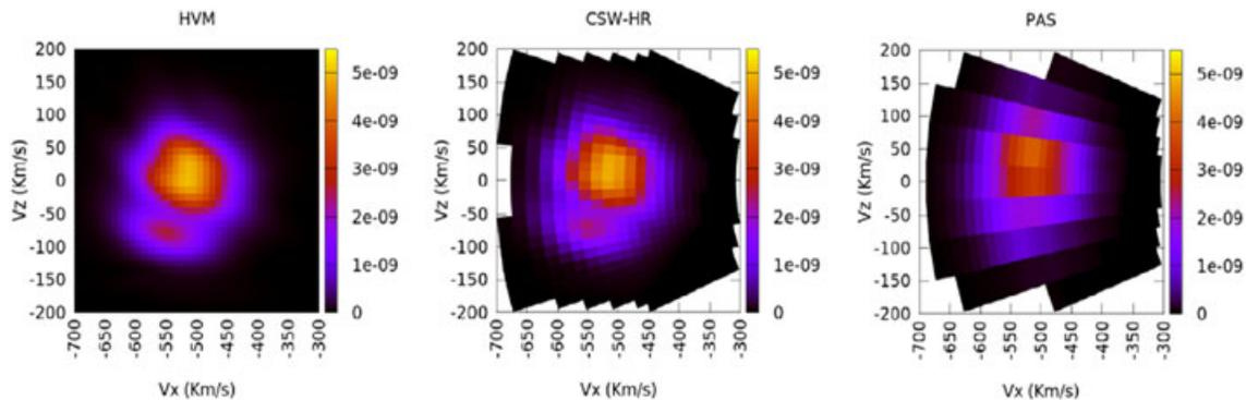
**Figure 14.** Illustration of the expected measurements of the proton distribution function on the basis of solar wind simulations described in DeMarco et al. [2016], respectively for the properties of (a) the simulation itself [Valentini et al., 2007], (b) the present design (THOR CSW instrument), and (c) the Solar Orbiter PAS instrument. The data are represented in a system equivalent to geocentric solar equatorial coordinates.
