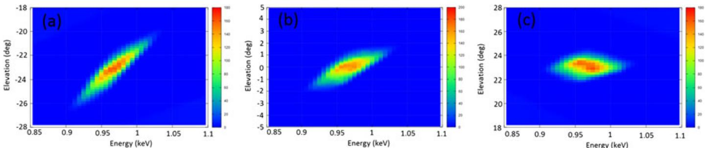
**Figure 6.** Response function calculated with SIMION showing the transmission rate over the energy and elevation response for three deflector potentials considered: (a)  $U_{def} = -170\text{ V}$ , (b)  $0\text{ V}$ , and (c)  $170\text{ V}$ . For this simulation both deflectors are polarized in an antisymmetrical fashion.
