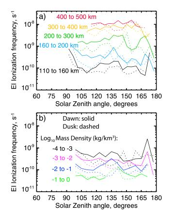
**Figure 5.**  $CO_2$  electron impact ionization frequency as a function of solar zenith angle is plotted separately for dawn (solid lines) and dusk (dashed lines), for five different altitude ranges (colors, top panel) and four different mass density ranges (colors, bottom panel).
