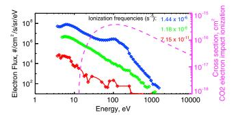
**Figure 1.** Example calculation of electron impact ionization frequency producing  $\mathrm{CO_2}^+$  ions. Blue, green, and red are three typical electron flux spectra seen on the Martian nightside. Electron impact ionization frequency is the integral over energy of the product of these spectra with the cross section (pink).
