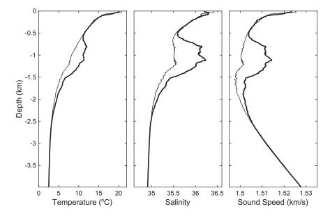
**Figure 6.** Temperature, salinity, and sound speed derived from nearby CTD casts obtained during the deployment of CAMBIOS moorings. A Meddy (thick line) was observed at 35.7597°N, 23.9429°W, while a CTD cast about 150 km away (thin line) at 34.2499°N, 21.7502°W measured no Meddy signature. The Meddy had temperatures about 3°C warmer, salinities about 0.6 ppt greater, and sound speeds 10–14 m s<sup>-1</sup> faster than ambient water.
