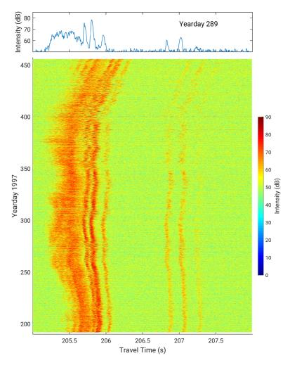
**Figure 3.** Acoustic receptions obtained along the T1–T2 acoustic path. The profile of a reception on yearday 289 is given in the top. About seven stable ray arrivals are evident, including a doublet arrival that appears in the top the largest amplitude peak and the three late-arriving bottom-reflected rays.
