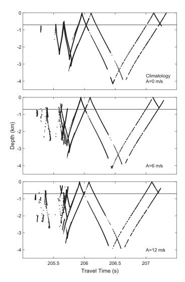
Figure 14. (top) Timefront for WOA09, as in Figure 9. (middle) Timefront for WOA09 plus a Meddy of 6 m s<sup>-1</sup> maximum sound speed. (bottom) Timefront for WOA09 plus a Meddy of 12 m s<sup>-1</sup> maximum sound speed. A Meddy along the acoustic path shifts the arrival pattern earlier and creates additional early arrivals.
