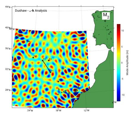
Figure 17. A snapshot of mode-1,  $M_2$  internal tides for the CAMBIOS region derived from the empirical model of Dushaw (2015). The internal tide field is a complicated interference pattern. The black segment indicates the T1–T2 acoustic path.
