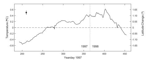
**Figure 20.** Temperature relative to the time-mean temperature estimated from the identified-ray travel times. The estimated temperature is an average over the range of the path and over 0–2,000 m depth interval. The formal inverse uncertainty is about 0.07°C as indicated at top left. The temperature variations can be mostly accounted for by latitudinal variations in the Azores Current. The scale at right indicates the approximate equivalent changes in latitude.
