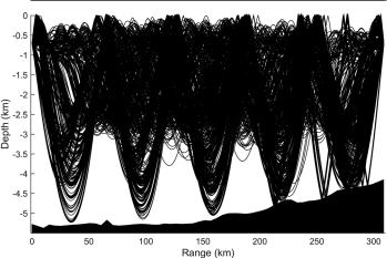
**Figure 15.** (top) Unperturbed ray paths, (middle) ray paths with hypothetical Meddy, and (bottom) ray paths with stochastic spice from Mediterranean water. A single sound speed section is used to compute the rays for each figure.
