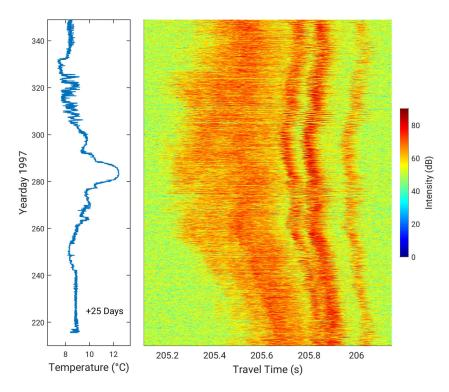
**Figure 19.** Close-up view of the measured acoustic travel time patterns during (right) the time of expected Meddy influences, compared to (left) the time variation of temperature observed on mooring T3. The latter time series was delayed by 25 days, roughly the length of time it would take a Meddy to travel from the mooring to the acoustic path.
