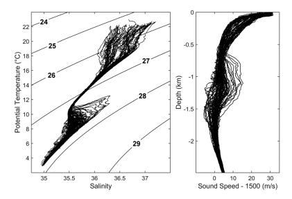
**Figure 10.** (left) *T–S* diagrams for 80 CTD casts and obtained during the deployment cruise for CAMBIOS in the Canary Basin (Figure 5). Values are for depths between the surface and 2.5 km. Contour values for sigma-*t* are shown to illustrate the variations of temperature and salinity along isopycnals. (right) Sound speed profiles associated with those casts. The significant influences of the spice of Mediterranean water on sound speed are obvious.
