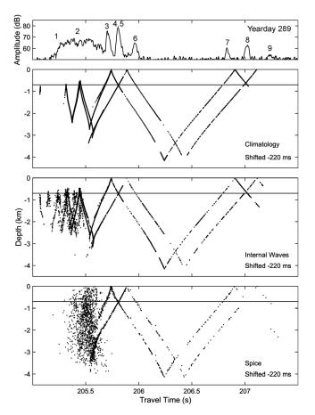
**Figure 9.** (top) Average arrival pattern for acoustic data obtained on yearday 289, 1997. Nine rays were tracked, as indicated. (top middle) Timefront for WOA09. (bottom middle) Timefront for WOA09 plus a single realization for internal waves. (bottom) Timefront for WOA09 plus spice.
