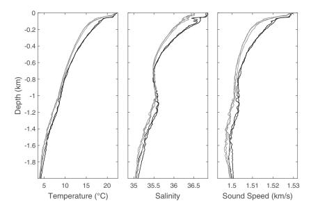
**Figure 7.** Five profiles of (left) temperature, (middle) salinity, and (right) sound speed obtained from CTD casts along the CAMBIOS T1–T2 tomography path during the deployment cruise. The path crossed the Azores Current which separates Western (18°C, black lines) from Eastern (15°C, gray lines) Atlantic water.
