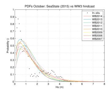
**Figure 6.** Scaled histogram of observed in situ wave heights during the Sikuliaq cruise (black dots), compared with Weibull distributions of the hindcast wave heights throughout the domain for October of the years 2007 through 2014 (colored curves). Hindcast from Thomson et al. (2016).
