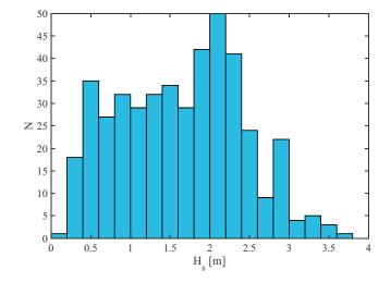
**Figure 7.** Histogram of wave heights observed remotely using the TerraSAR-X satellite system during October 2015.
