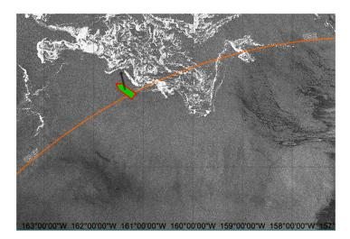
**Figure 3.** Example RADARSAT-2 image with ship location (green symbol). The orange line is the boundary of the US Exclusive Economic Zone (200 nm from the coast). RADARSAT-2 data and products from MacDonald, Dettwiler, and Associates Ltd., All Rights Reserved.
