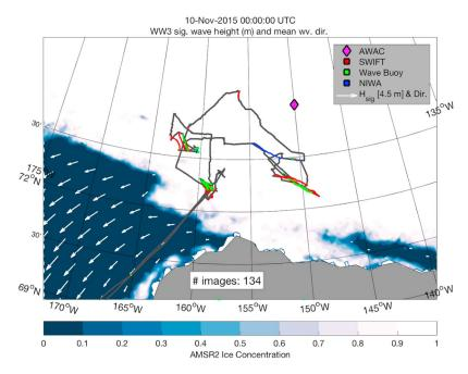
**Figure 2.** Map of cruise track and buoy deployments, overlaid on the ice and wave conditions at the end of the experiment. This is the final frame of a movie, which is included as supporting information S1, showing the progression of the entire research cruise.
