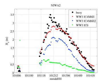
**Figure 11.** Wave height time series during Wave Experiment 3. Black dots are observations from the NIWA buoy. Colored dots are from a WAVEWATCH III hindcast using the original ice parameterization (green) and newly implemented ice parameterizations (red, blue).
