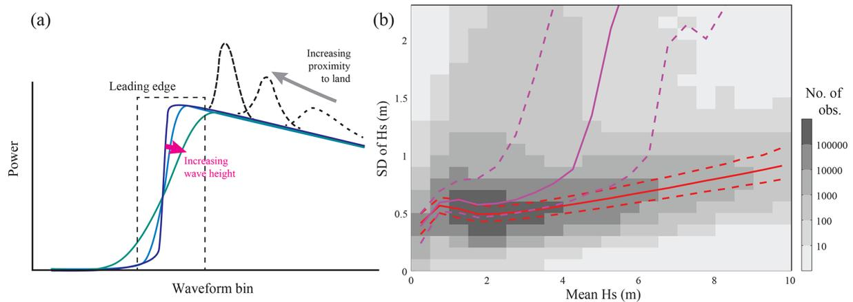
**Figure 16.** (a) Schematic of how conventional waveforms are affected by varying wave height and proximity to land. (b) Variability within a 1 s ensemble as a function of mean conditions. Illustration is from the default retracker for JASON-3, with grey shading indicating the population density for open-ocean conditions and the red lines indicating the 25th, 50th, and 75th percentiles for 0.5 m wide bins. Pink lines show the same analysis for points within 15 km of the coast.
