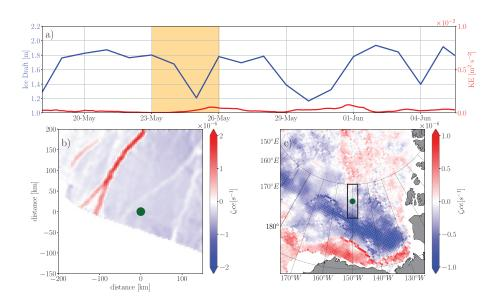
**Figure 4.** Time series of ice draft (blue) and KE (0–30 m, red) from the ADCP in 2018 (a). The orange box in (a) shows the period of interest between May 23–26. Average of sea ice vorticity from three pairs of SAR images (b) and from NSIDC (c) for May 23–26, 2018. The green dot is the position of the mooring and the black box in (c) indicates the window of (b).
