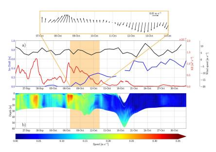
**Figure 2.** (a) Time series of ice draft (blue), KE (0–30 m, red) from the Acoustic Doppler Current Profiler (ADCP) and wind speed (black) in 2017. A stick diagram of the ocean current anomalies (relative to the mean over October 7–13) is shown in the orange box. (b) Ocean speed profiles from the ADCP.
