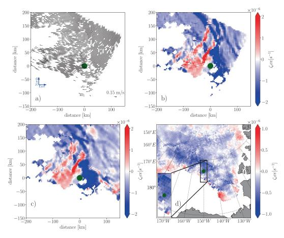
**Figure 3.** (a) Sea ice drift field and (b) sea ice vorticity from one pair of SAR images for October 12–13; (c) average of sea ice vorticity from five pairs of SAR images for October 7–13 and (d) from the National Snow and Ice Center (NSIDC) for October 7–13. The green dot indicates the position of mooring B, and the black box indicates the window of (a, b, and c).
