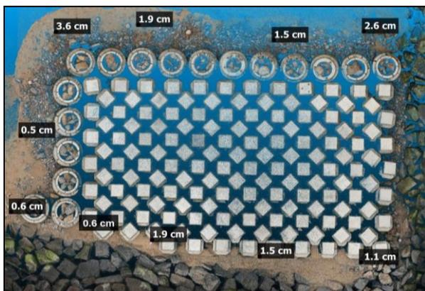
**Figure 7.** Georeferencing errors on each of the ten targets
