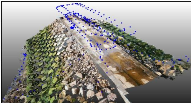
**Figure 18.** Photogrammetric model of the dike in Cherbourg
