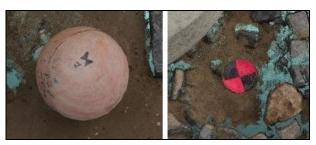
Figure 5. Spherical (on the left) and flat (on the right) targets
