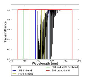
**Figure 1.** 3MI's filter models. The  $O_2$  transmittance is indicated by the black line. The green line represents the out-band filter (748.95–753.25 nm), the red the broad-band (745–785 nm), the blue 3MI's in- or thin band (758–768 nm), and the yellow line MSPI's in-band (762.5–764.9 nm).
