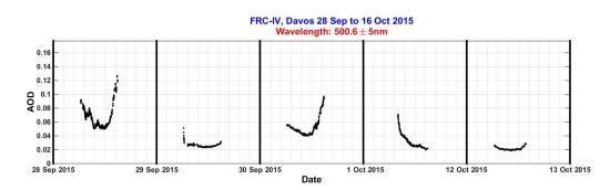
Figure 1. Average AOD at 500 nm measured by the three reference PFR instruments (WORCC triad) during 5 days with cloud-free sky conditions. Data points represent 1 min measurements.
