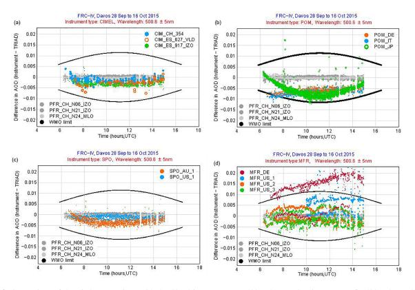
**Figure 2.** Comparison of the triad (gray points) with the Cimel instruments ( $\mathbf{a}$ , 500 ± 5 nm), POM instruments ( $\mathbf{b}$ , 500 ± 5 nm), SPO instruments ( $\mathbf{c}$ , 500 ± 5 nm) and with the MFR instruments ( $\mathbf{d}$ , 862 ± 5 nm). Different colors represent different instruments for all the five comparison days, and gray lines represent the WMO AOD limits.
