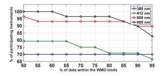
Figure 5. Percentage of instruments that lie within the WMO criterion (0.005 + 0.01/m optical depths). The horizontal axis shows the different percentages of measurements within the criterion ending at 95 %, which is the U95 WMO limit.
