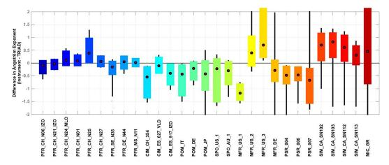
**Figure 6.** Difference in the Ångström exponent between each instrument and the WORCC triad. The boxes represent the 10th and 90th percentiles, while the black lines represent the minimum and maximum values of the distribution excluding the outliers. Outliers (gray dots) are considered to be values outside the 10th and 90th percentiles by 4 times the width of the distribution at a 10 % level. Box colors are only used to differentiate between instruments.
