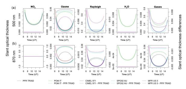
Figure 9. Slant column optical thickness (right axis – thick lines) and optical depth differences compared with the triad (left axis dashed lines), at 500 (a) and 870 nm (b).
