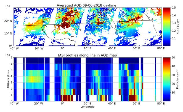
Figure 4. Cross section of MAPIR dust profiles on 9 June 2018. The first plot gives a map of the retrieved daytime  $10 \,\mu m$  AOD on a  $0.5^{\circ}$  by  $0.5^{\circ}$  grid over the region we are interested in. The black line represents the locations along which the cross section in the second plot is given. Each profile of the cross section is an average of all profiles within  $0.5^{\circ}$  of the transect line.
