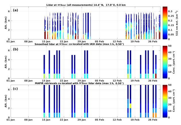
**Figure 8.** Mineral dust profile comparison at M'Bour site (Senegal) from 1 January to 1 March 2015. Panel (a) gives the lidar data (extinction profiles at 532 nm) as provided for this study. In panel (b), the lidar data smoothed according to Eq. (7) are presented, for those times when there is a co-located MAPIR profile. Panel (c) presents the MAPIR profiles over time averaged around the M'Bour site.
