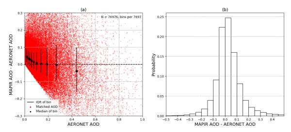
**Figure 7.** MAPIR AOD, converted to 550 nm, versus the AERONET SDA coarse-mode AOD difference distribution. (a) Scatter plot of the AOD difference in function of the AERONET AOD (red dots), for all considered stations combined. Data are split into 10 bins of equal quantity; corresponding binned median (black dots) and interquartile range (IQR, vertical black lines) are shown. (b) AOD difference histogram.
