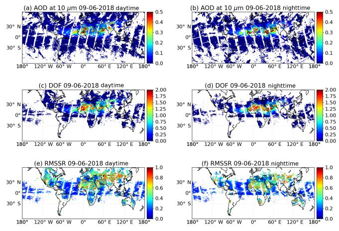
Figure 3. (a, b) Maps of the aerosol optical depth (AOD) at 10 µm on 9 June 2018, calculated by integrating the retrieved aerosol profiles and multiplying them by the extinction cross section. (c, d) Maps of the degrees of freedom (DOF), June 2018. (e, f) Maps of the root mean square of the spectral residuals (RMSSR). Daytime (nighttime) measurements on the left (right) correspond to a mean local solar time of 09:30 (21:30) when crossing the Equator.
