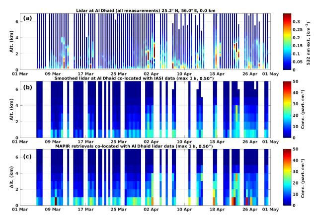
**Figure 10.** Mineral dust profile comparison at the Al Dhaid site (UAE) from 1 March to 1 April 2018. Panel (a) gives the lidar data (extinction profiles at 532 nm) as provided for this study. In panel (b), the lidar data smoothed according to Eq. (7) are presented, for those times when there is a co-located MAPIR profile. Panel (c) presents the MAPIR profiles over time averaged around the Al Dhaid site.
