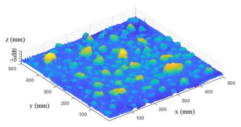
Fig. 2 – 2.5D DEM of second laboratory soil surface with high clod concentration at initial stage.
