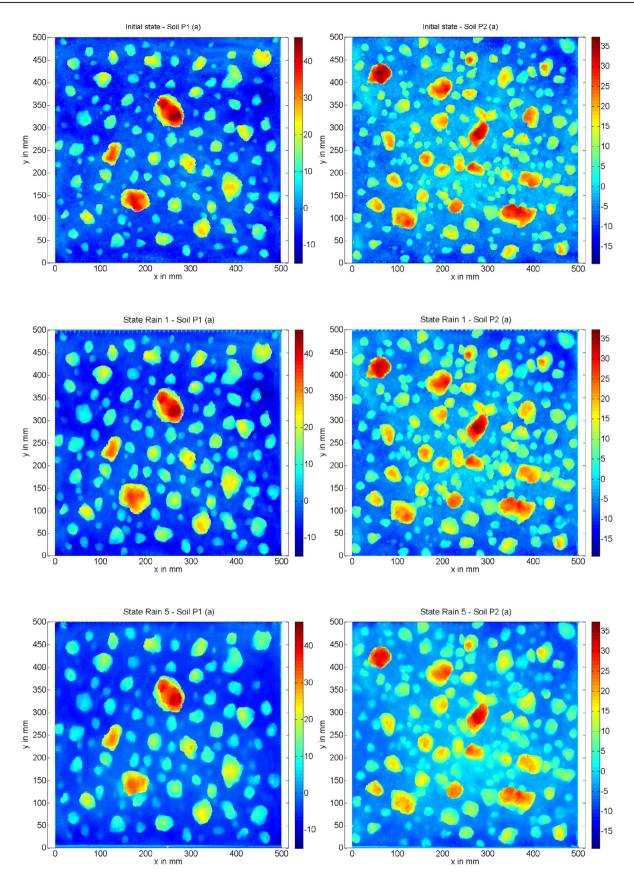
Fig. 1 — Top view of soil surfaces under study at initial state (top row), after first rainfall (middle row), after last rainfall (bottom row). Laboratory made soil surfaces with a low clod concentration (left column) and, with a high clod concentration (right column).
