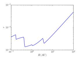
Figure 6. Dimensionless cooling time as a function of radius in a  $0.01 \, M_{\odot}$  disc model. Jumps are due to the condensation of molecules on to dust grains which abruptly change opacities (Semenov et al. 2003).
