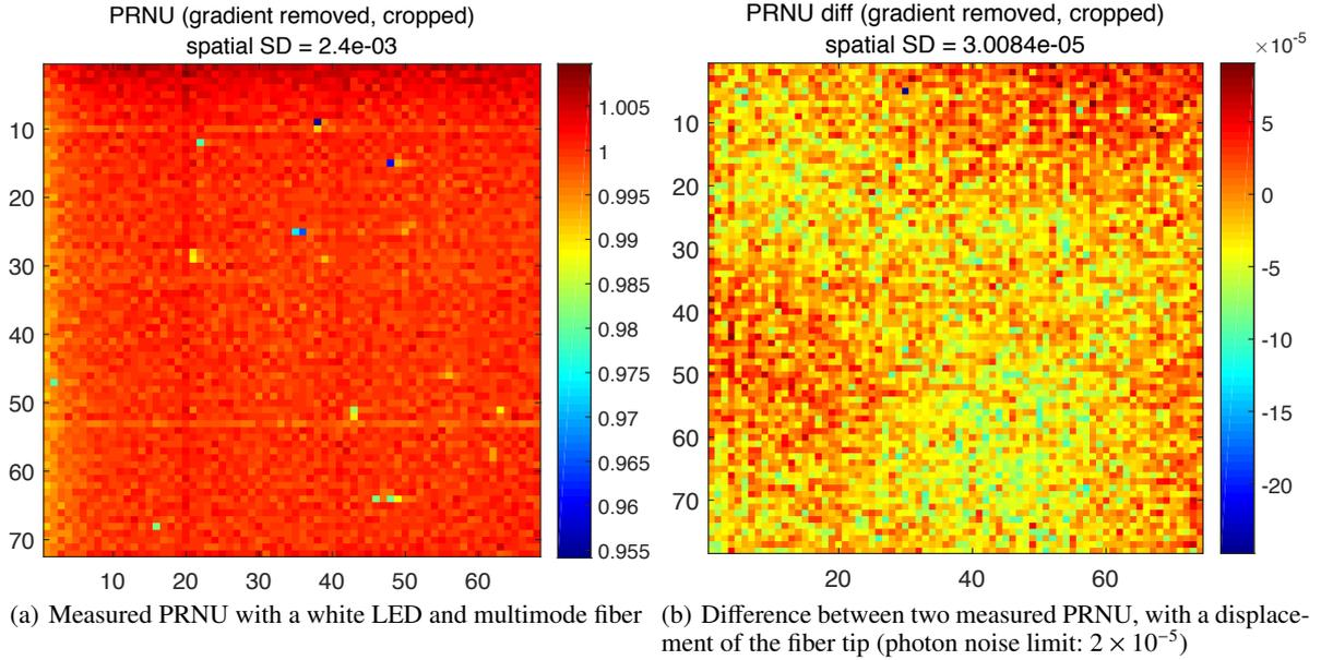
**Fig. 16.** PRNU and its difference with a displacement of the fiber tip.
