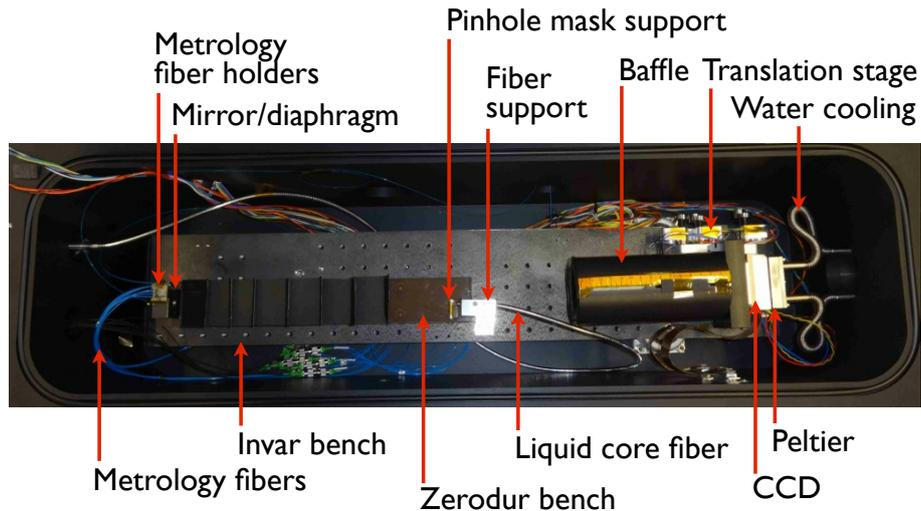
**Fig. 4.** Optical bench inside the vacuum chamber.
