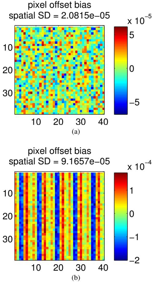
**Fig. 14.** Pixel offsets bias (in the horizontal direction) for different PRNU RSD. The maps show the difference between the pixel offsets found after processing and the solution of the simulation, for PRNU RSD of  $5 \times 10^{-5}$  **a)**, and  $2 \times 10^{-3}$  **b)**. The residuals for **a)** are at the photon noise floor, while a stronger systematic bias of  $1 \times 10^{-4}$  pixel is visible for **b)**. Both have the same photon noise.
