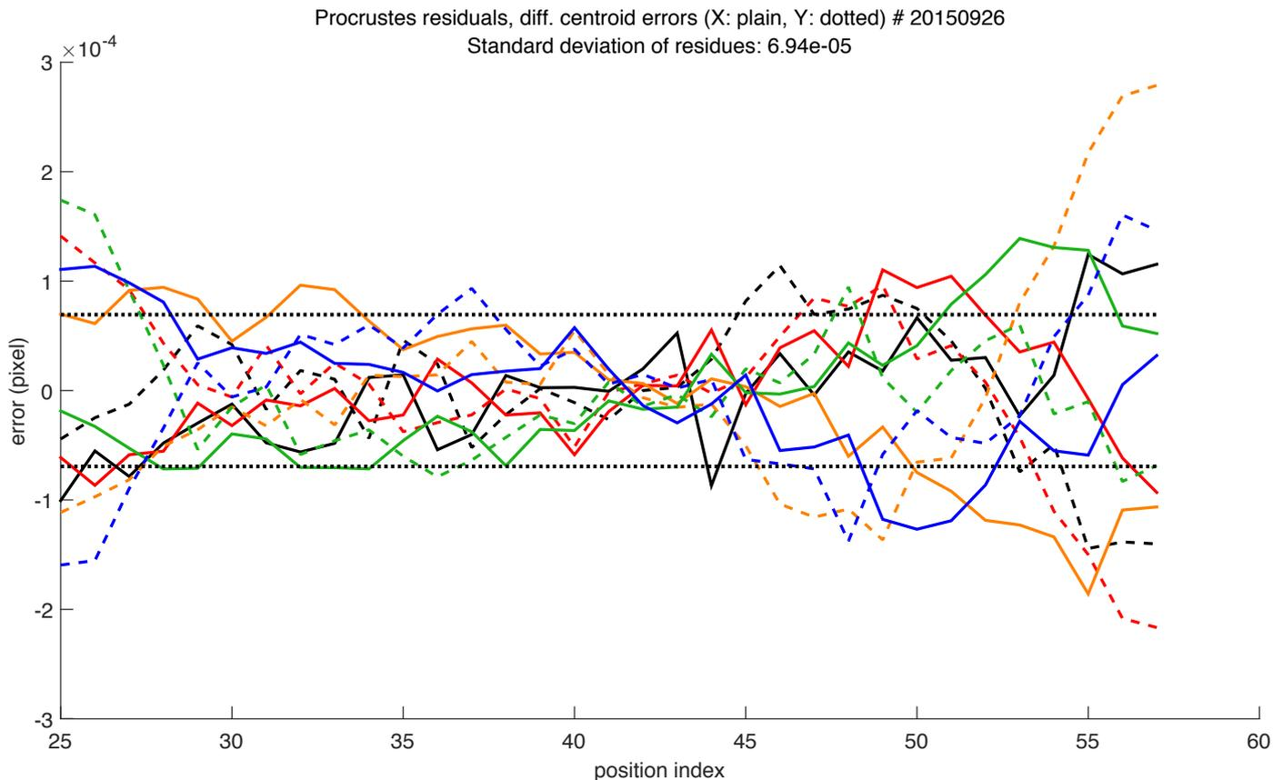
**Fig. 23.** Procrustes residuals for each position (from index 25 to 57). In this case the PRNU and pixel offset calibration are used. Each centroid has a different color (black centroid is the central one). The horizontal dotted lines indicate the dispersion of the residues ( $\pm\sigma$ ).
