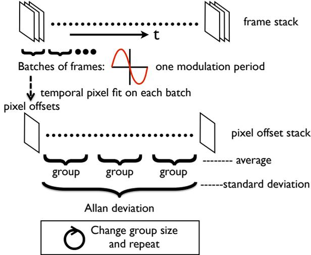
**Fig. 10.** How to calculate the Allan deviations.
