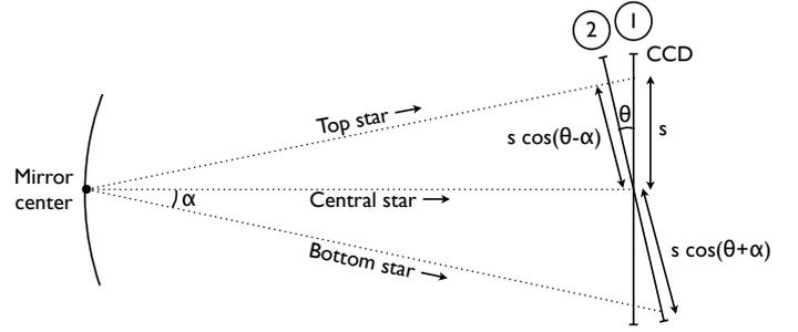
Fig. D.1. Illustration of the non-homogeneous projection effect.
