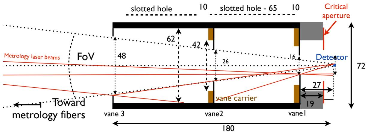
Fig. 7. Schematic of the baffle. The dimensions are proportional (indicated in mm). The red rays coming from the left are from the metrology fibers. Only the most geometrically constraining rays are represented.
