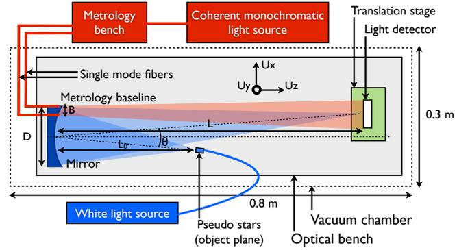
**Fig. 2.** DICE testbed concept (top view, not to scale). The elements associated with the metrology, the pseudo stars and the mechanical supports are respectively in red, blue and grey. The  $(X, Y, Z)$  axis indicated on the figure will be used consistently throughout the paper to indicate directions.
