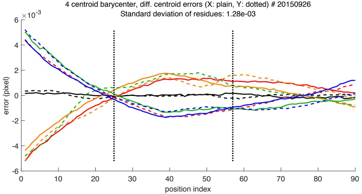
**Fig. 22.** Barycenter residuals for each position (from index 1 to 90). Each centroid has a different color (black for the central one). Plain lines are X axis residuals, dotted lines are Y axis residuals. Indexes between 25 to 57 (final dataset for accuracy) are indicated by the vertical dotted lines.
