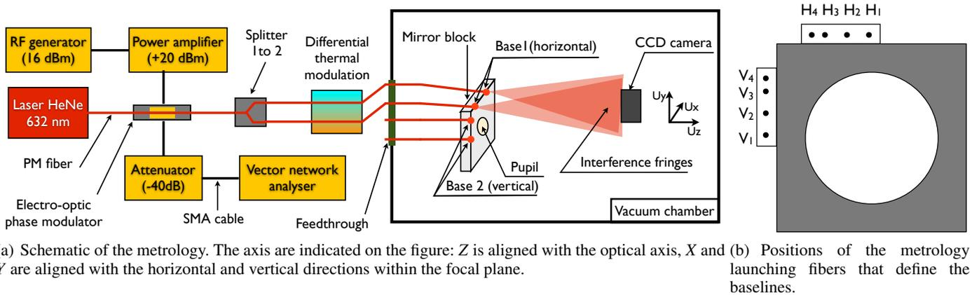
Fig. 6. The metrology subsystem.
