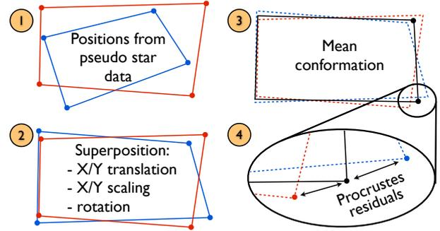
**Fig. 11.** Diagram of the Procrustes analysis. The relative centroid positions for two geometric conformations, each corresponding to one detector position, are represented respectively in red and blue. The black conformation (plain black line at step 3) is the average between the red and the blue ones.
