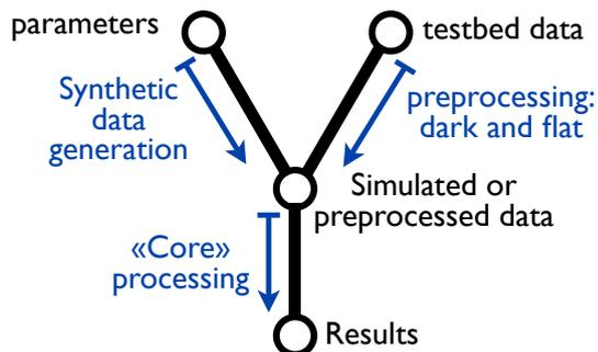
**Fig. 12.** Actual data and synthetic data flow diagram. The pseudo star and metrology data analysis scripts both follow this architecture. An option setting parameter can be used to switch between synthetic and actual data.
