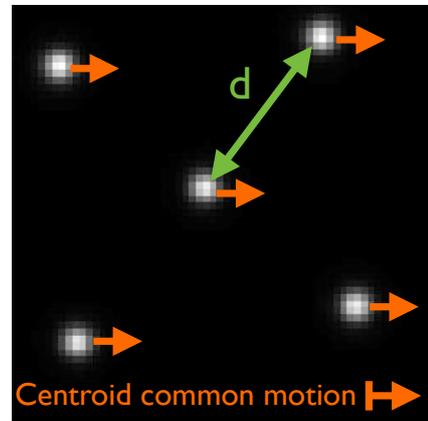
**Fig. 3.** Simplified experiment principle. The orange arrows represent the CCD motion, which appear as a common motion of all centroids. The final astrometric accuracy is measured as the standard deviation of the distance. The location of each centroid is measured by “autocorrelation after resampling by Fourier transform”.
