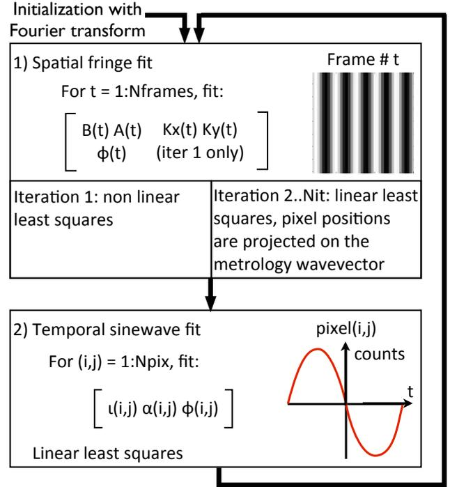
**Fig. 9.** Iterative process used to fit the metrology fringes (step 2 in Fig. 8). The difference between the measured phase of a pixel ( $\phi(i, j)$ ) and the phase expected (global fringe phase) is the phase offset caused by the pixel offset projected in the direction of the wavevector.
