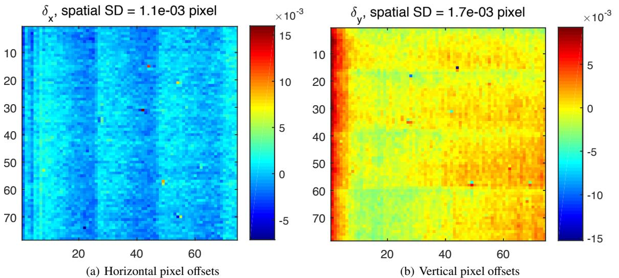
**Fig. 17.** Pixel offsets (in pixel units) as measured by the metrology (baseline H1H4-V1V4).
