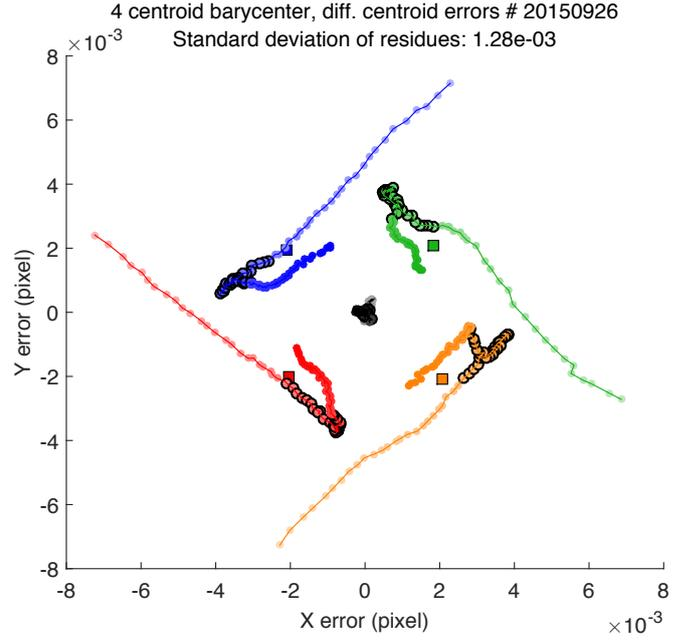
**Fig. 21.** Barycenter residuals for each position (from index 1 to 90). Each centroid has a different color (black centroid is the central one). The relative positions between pseudo stars (illustrated by the squares) have been downscaled to correspond to the magnitude of the residuals. Indexes between 25 to 57 (final dataset for accuracy) are circled in black.
