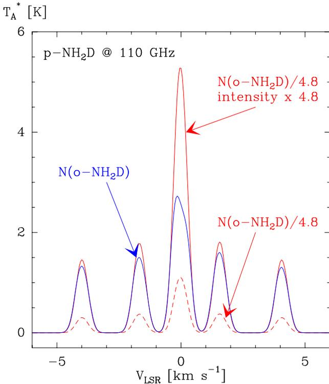
**Figure 7.** Models for the  $\text{p-NH}_2\text{D}$  110 GHz transition. The blue curve gives the intensity we would obtain with a  $\text{p-NH}_2\text{D}$  abundance profile identical to that of  $\text{o-NH}_2\text{D}$ . The red dashed curve corresponds to the model adopted to reproduce the  $\text{p-NH}_2\text{D}$  110 and 494 GHz lines, with an OPR of 4.8. The red curve corresponds to the same model with the intensity multiplied by a factor 4.8.
