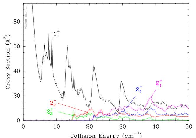
**Figure 3.** Cross sections for  $o\text{-ND}_3$  that originate from the  $1_1^-$  level. This figure can directly be compared to fig. 13 of Ma et al. (2015) and the cross-sections obtained in the latter study are reported as dotted lines.
