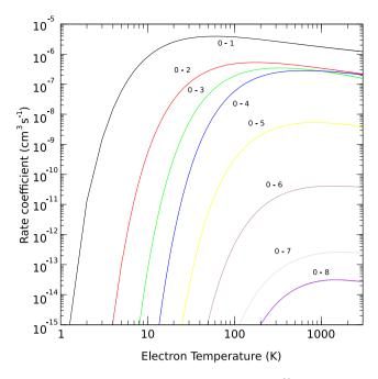
**Figure 6.** Rate coefficients for rotational excitation of  $^{38}$ ArH<sup>+</sup> from the ground state (J = 0) to the lowest eight excited states.
