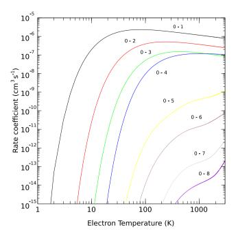
**Figure 3.** Rate coefficients for rotational excitation of CH<sup>+</sup> from the ground (J = 0) state to the lowest eight excited states.
