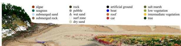
Figure 8. Extract of the resulting 3D classification: the sandy dune of Sables d'Or les Pins and its surroundings.
