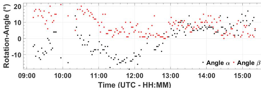
Fig. 6. Rotation angles for the alignment of the lander rotation axis relative to the lander z-axis for individual 20 min intervals overlapping by 90%. Fewer data points are available around 10:20 UTC due to external magnetic field conditions.
