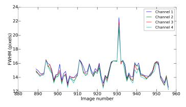
Fig. 1. FWHM in different images. Each line represents a different qPDI channel.
