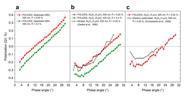
**Figure 2.** Measurements of (a) Spectralon with and without depolarizer, (b) surface made of 3-μm-diameter aluminum oxide (WCA3) with and without depolarizer and as measured by Geake and Geake (1990), and (c) same surface measured with depolarizer at 625 nm compared to measurement by Ovcharenko et al. (2006) at 630 nm. The red phase curves are available in Data Set S1. POLICES = POLarimeter for ICE Samples.
