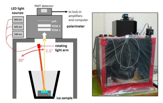
**Figure 1.** The POLarimeter for ICE Samples setup, consisting of a hermetical enclosure allowing the measurements of photometric and polarimetric phase curves of icy samples under dry and cold conditions. A motorized "light arm" illuminates the sample surface with monochromatic light at incidence angles from 1.5° to 30°, and a polarimeter analyzes the scattered light at a fixed emergence of 0°. LED = light-emitting diode; PEM = photoelastic modulator.
