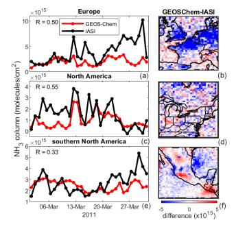
**Figure 8.** (**a**, **c**, **e**) Time series of daily NH<sub>3</sub> columns derived from IASI (black lines) and the GEOS-Chem model (red lines) over Europe (**a**), North America (**c**), and southern North America (**e**). (**b**, **d**, **f**) Maps of NH<sub>3</sub> columns (in molec.  $\text{cm}^{-2}$ ) differences between IASI and GEOS-Chem model (model observations) for March 2011.
