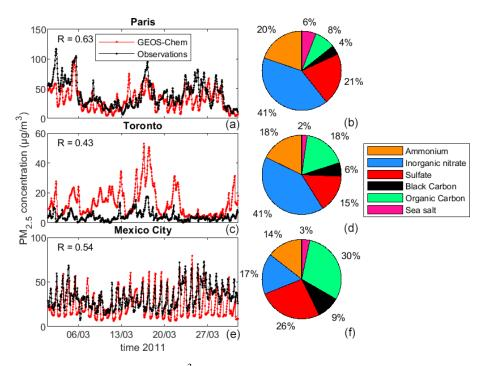
**Figure 9.** (**a**, **c**, **e**) Time series of hourly  $PM_{2.5}$  ( $\mu g m^{-3}$ ) derived from surface observations (black lines) and the GEOS-Chem model (red lines) over Paris (**a**), Toronto (**c**), and Mexico City(**e**) for March 2011. (**b**, **d**, **f**)  $PM_{2.5}$  speciation (% in total mass) derived from the GEOS-Chem run for March 2011.
