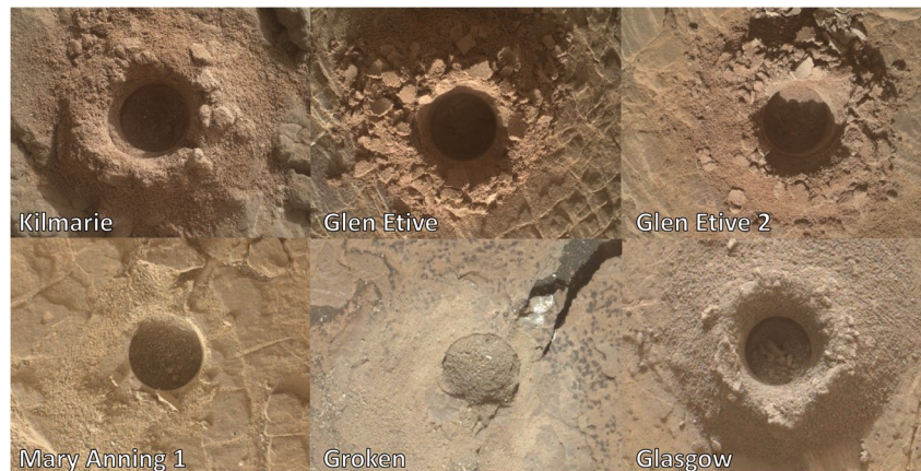
Figure 3. Mars Hand Lens Imager (MAHLI) images of the Glen Torridon drill holes from which the samples discussed here were obtained. Each hole is approximately 1.6 cm in diameter. Kilmarie (MAHLI image: 2404MH0007740010900288C00) was drilled from the Jura member. Glen Etive (2524MH0007740010903140C00), Glen Etive 2 (2550MH0007740010903254C00), Mary Anning (2851MH0001970011003289C00), and Groken (2920MH0004240011003512C00) were drilled from the Knockfarril Hill member. Glasgow (2773MH0004240011002826C00) was drilled from the Glasgow member. NASA/JPL-Caltech/MSSS.
