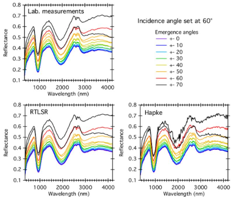
*Fig. 1: Bidirectional reflectance spectroscopy of the howardite measured in the laboratory (top left panel), and simulations based on inversion with the RTLSR model (bottom left panel) and with the Hapke model (bottom right model).*
