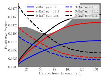
**Figure 6.** Polarization fraction as a function of distance from the center of our modeled debris disk. Solid lines show results for *k*-RAT alignment. Dashed lines show results for *B*-RAT alignment. Different colors represent dust grains with different values of the intrinsic polarization fraction  $p_0$ . The shaded region is the region permitted by our ALMA observations; the upper envelope of the region is the same as the curve shown in the right-hand panel of Figure 3.
