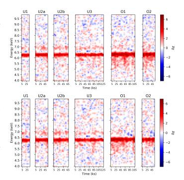
**Fig. A.1.** RMs produced using a power law plus total covering cold absorption fitted only in the 4–5 keV and 7–10 keV energy bands, following the indications of Tombesi et al. (2007). The value of the column density of the absorber is fixed to the value measured in average spectra in top panel maps and free to vary in the bottom panel ones.
