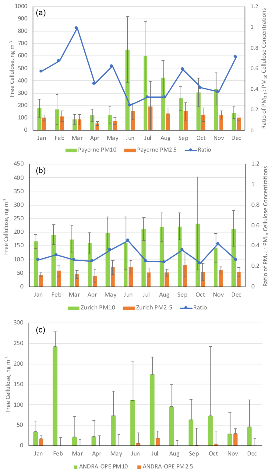
Figure 3. Monthly averages of cellulose concentrations within PM 10 (green bars) and PM 2.5 (orange bars) at the three sampling sites of Payerne (rural, a ), Zurich (urban, b ), and ANDRA-OPE (rural, c ). Black error bars represent 1 standard deviation of the results. The corresponding blue lines represent the ratio of the monthly mean cellulose concentrations in PM 2.5 : PM 10 . Note that ANDRA-OPE data are only for the year of 2020, and only positive error bars are used for clarity (SD larger than mean).
