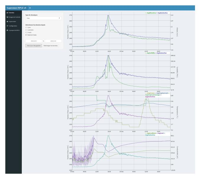
**Figure 8.** Screenshot of the "Data visualization" menu of the user interface in the default mode. Four time series graphs are displayed from top to bottom: (1) water level and surface water velocity, (2) water level and turbidity, (3) water level and temperature, and (4) water level and conductivity.
