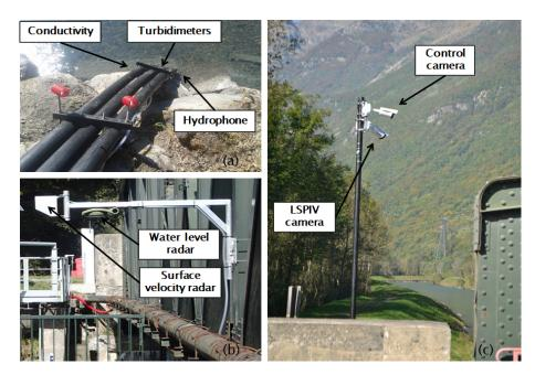
**Figure 4.** Photos illustrating the deployment of instruments in situ (a) submerged instruments (conductivity probe, turbidimeters and hydrophone) housed in the polypropylene tubes anchored to the river bank; (b) water level and surface velocity radars supported by extensible brackets fixed to the bridge parapet; (c) control digital camera and LSPIV digital camera fixed at the top of a mast located on the river bank.
