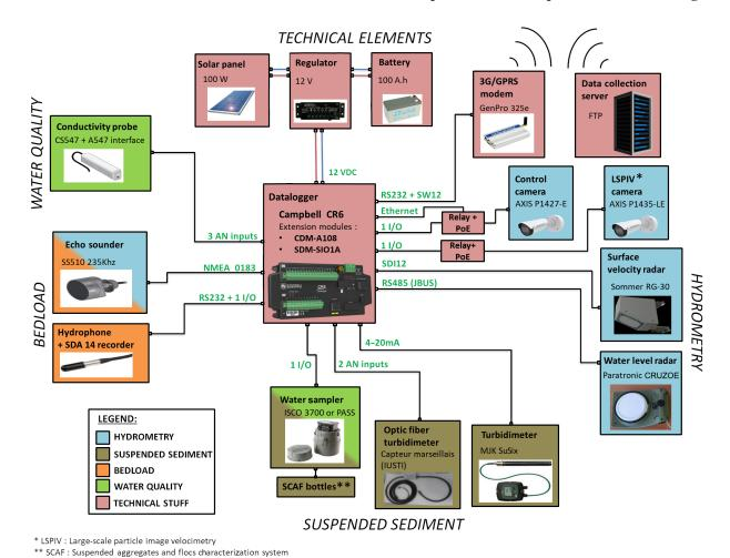
**Figure 2.** The RIPLE platform architecture.
