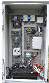
**Figure 3.** Photos of the box that houses all the electronics of the platform and the battery: (a) outside view where we also see the solar panel and the ISCO automatic river water sampler and (b) inside view.
