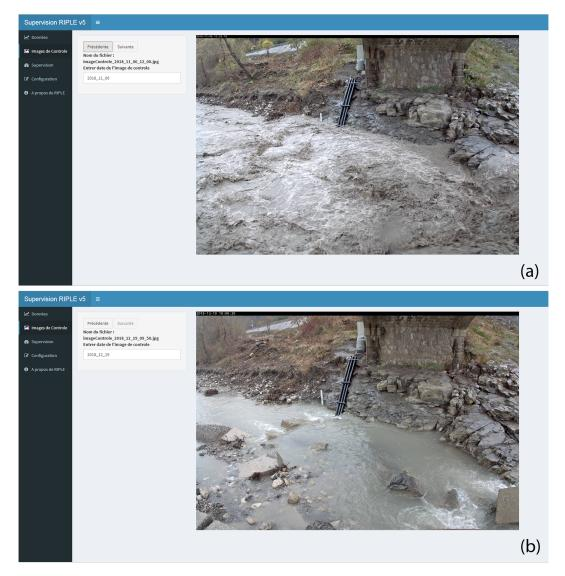
Figure 10. Screenshots of the "Images of control" menu of the user interface at two dates: (a) 6 November 2018 12:00 UTC during a flood and (b) 19 December 2018 10:00 UTC for low-water conditions.
