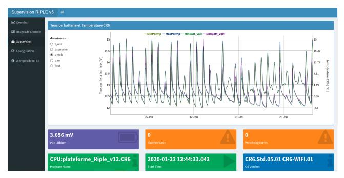
**Figure 11.** Screenshots of the "Supervision" menu of the user interface. A time series graph is displayed with minimum and maximum battery voltage on the first *y* axis and min and max air temperature on the second *y* axis.
