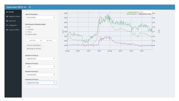
**Figure 9.** Screenshot of the "Data visualization" menu of the user interface in the personalized mode. A graph can be created with two variables on the first y axis and two variables on the second y axis, with time on the x axis. In this case, the water level, water surface velocity and distance measured by the echo sounder are displayed.
