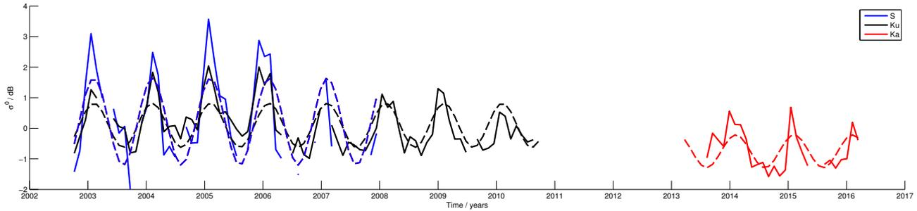
**Figure 1.** Time series of the backscattering coefficient at the S (blue), Ku (black) and Ka (red) bands at location (69.468° S, 134.28° E) between October 2002 and December 2007 at S band, October 2002 and September 2010 at Ku band and March 2013 and March 2016 at Ka band. The dashed lines represent the best fits to the time series (see Eq. 1). The observations show the seasonal cycle with a 1-year period at the different frequencies.
