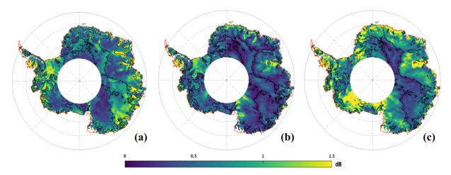
**Figure 5.** Spatial distribution of the seasonal amplitude of the backscattering coefficient at the S (a), Ku (b) and Ka (c) bands. Black contour lines delineate regions where the backscattering coefficient at the Ku band peaks before April. The cross mark represents the location of the time series shown in Fig. 1. White areas indicate regions where no observations are available (latitudinal orbit limit of 81.5° S). Values are expressed in dB.
