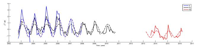
**Figure 1.** Time series of the backscattering coefficient at the S (blue), Ku (black) and Ka (red) bands at location (69.468° S, 134.28° E) between October 2002 and December 2007 at S band, October 2002 and September 2010 at Ku band and March 2013 and March 2016 at Ka band. The dashed lines represent the best fits to the time series (see Eq. 1). The observations show the seasonal cycle with a 1-year period at the different frequencies.
