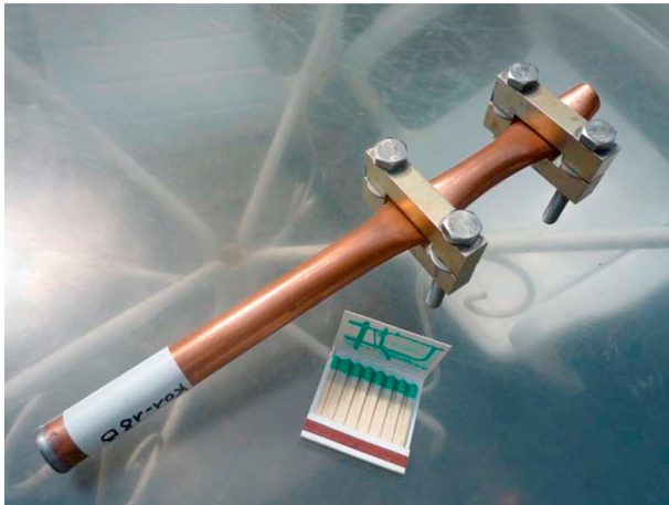
Figure 2. Copper tube (1 inch diameter) equipped with two clamps, used for storing the ice sample.
