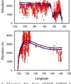
Figure 5. Elevation data from ASTER GDEM V3 (red) extracted along an ICESat L3J laser altimetry profile for two segments of Track 1305 (blue). A profile for L3K offset by 200 m is shown in black.
