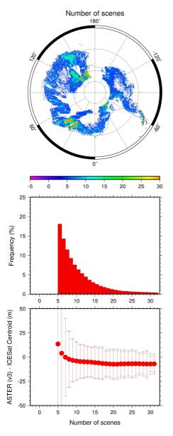
Figure 9. Geographic distribution of  $5 \le N < 31$ , frequency distribution, and means, standard deviations and RMSEs for the edited data in Antarctica (bottom right).
