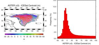
Figure 2. Map of ASTER GDEM V3 – ICESat elevation differences in meters for all available GCPs from Laser 3 in Greenland (left), and frequency distribution (%) of the differences (right).
