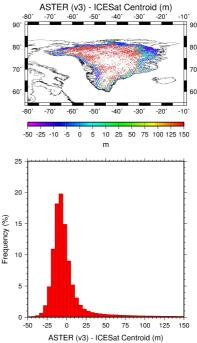
Figure 10. Geographic distribution of ASTER GDEM V3 minus ICESat elevation differences (top) for edited data ( $5 \le N < 31$ ) and their frequency distribution (bottom) in Greenland, corresponding to the statistics displayed in Figure 8.
