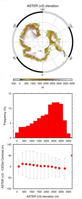
Figure 15. Map of ASTER GDEM V3 minus ICESat GCPs elevation differences (in meters) for Antarctica (top). Frequency distribution for data binned at 250 m (center), and means standard deviations and RMSEs of the differences (bottom).
