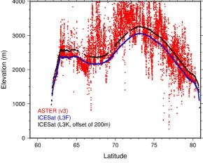
Figure 4. Elevation data from ASTER GDEM V3 (red) extracted along an ICESat L3F laser altimetry profile for Track 1290 (blue). A profile for L3K offset by 200 m is shown in black.
