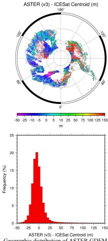
Figure 11. Geographic distribution of ASTER GDEM V3 minus ICESat elevation differences (top) for edited data ( $5 \le N < 31$ ) and their frequency distribution (bottom) in Antarctica, corresponding to the statistics displayed in Figure 9.
