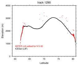
Figure 12. ASTER GDEM V3 edited profile ( $5 \le N < 31$ ) across the ICESat L3F profile (track 1290) in Greenland (see Figure 4 for the location on the map).
