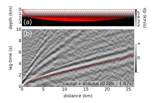
**Figure 7.** Comparison between the theoretical traveltimes predicted using ray tracing in the 1-D P wave velocity model for Soultz-sous-Forêts (a) and the noise correlation functions of the EstOF network (b). The causal and acausal sides from Figure 6a are band-pass filtered between 0.28 and 1.67 s (0.6–3.5 Hz) and averaged to highlight the P wave phase.
