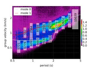
**Figure 11.** Position of the 15 clusters used in the period group-velocity domain. Numbers indicate the station pairs retained in each cluster. White (red) rectangles indicate clusters labeled fundamental mode (first overtone). Solid curves indicate the theoretical group velocity dispersion curves for the Soultz model.
