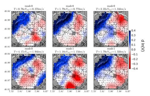
**Figure 12.** Rayleigh wave group velocity dispersion maps at several periods and for the fundamental mode (mode 0, a–d) or the first overtone (mode 1, e, f). The amplitudes correspond to velocity variations relative to a reference group velocity, specified in the subplot title of each map.
