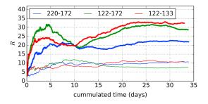
**Figure 4.** Convergence of the noise correlation function for three pairs of nodes in the EstOF network (220–172, 122–172, and 122–133). The ratio (R) between the peak amplitude in the direct arrival window (group velocity between 0.3 and 3.5 km/s) and the coda window (group velocity between 0.15 and 0.3 km/s) is measured for both causal (thick curves) and acausal sides (thin curves).
