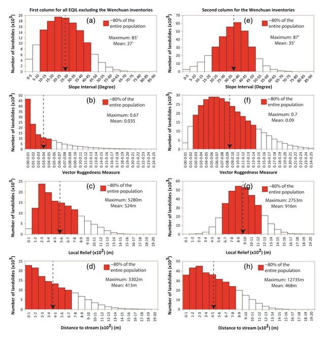
**Figure 5.** Frequency values of earthquake-induced landslides in intervals of (a) slope, (b) vector ruggedness measure (VRM), (c) local relief, and (d) distance to stream for all EQIL excluding the Wenchuan inventories (in first column), and for the (e–h) Wenchuan inventories separately (in second column). The arrows point out the mean values.
