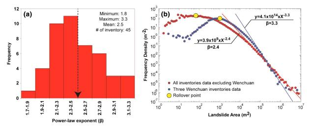
**Figure 7.** (a) Frequencies for estimated power law exponents for the EQIL inventories and (b) the frequency-density distributions for the landslides gathered from all inventories excluding the Wenchuan event (red) and the landslides gathered from the two Wenchuan inventories (blue). The arrow points out the mean value.
