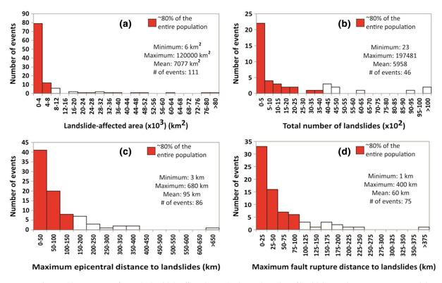
**Figure 4.** Frequency values and basic statistics for (a) the landslide-affected area, (b) the total number of landslides, (c) the maximum epicentral distance to landslides, and (d) the maximum fault-rupture distance to landslides. Red bars show the range of values for 80% of the total number of EQIL events in the database for which information was available. Since many inventories are not complete, in most cases, these refer to minimum values.
