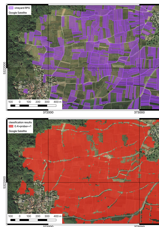
Figure 9. Comparison between the vineyard mapping on the subset 2 between the RPG database (above) and the Imclass results (below).
