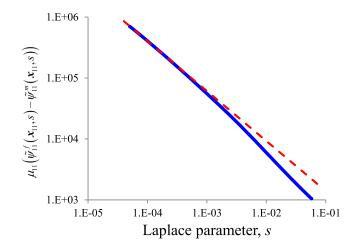
**Figure 3.** Blue (solid) curve: estimate of the fracture-matrix drawdown differential,  $\mu_{11}(\bar{\psi}_{11}^{\prime}(\mathbf{x}_{11},s)-\bar{\psi}_{11}^{\prime\prime}(\mathbf{x}_{11},s))$ , based on the data from the test depicted in Figure 2 and (9); red (dashed) line: best linear estimate (in log-log space) obtained using only data for small values of the Laplace parameter *s*, indicating a power law behavior.
