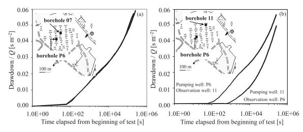
Figure 1. Drawdown curves observed during interference pumping tests performed at the Hydrogeological Experimental Site (HES): (a) example of reciprocity detected between wells P6 and 07; (b) example of observed reciprocity gaps between wells P6 and 11. Figure adapted from *Delay et al.* [2011].
