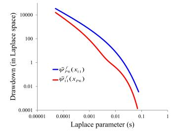
**Figure 2.** Discrete Laplace transform of the drawdown data observed at well 11 when pumping is performed at well P6 (in blue) and of drawdowns measured at P6 when pumping in 11 (in red). Curves are constructed by transforming the drawdown data depicted in Figure 1b to Laplace space.
