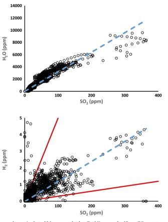
**Fig. 3**  $CO_2$ ,  $H_2O$ ,  $H_2S$  and  $H_2$  vs  $SO_2$  scatter plots of the mixing ratios in the El Misti plume. Measurements were taken on 1 December 2015 for 30 min at an acquisition frequency of 1 Hz. Least-square regression lines
