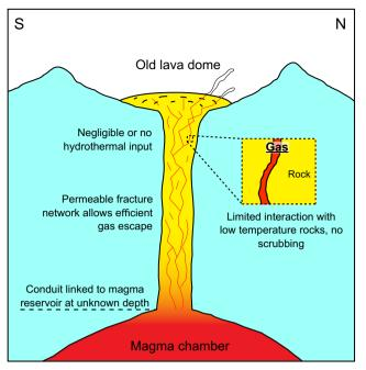
**Fig. 7** Schematic cross-section through the El Misti conduit highlighting the main conclusions from this study. Magmatic gases are released from a reservoir at unknown depth and quickly migrating to the surface through a network of established fracture with the conduit and lava dome. During ascent, the gas has very limited chemical interaction with the host rock and remains isolated from contamination by the surrounding hydrothermal system
