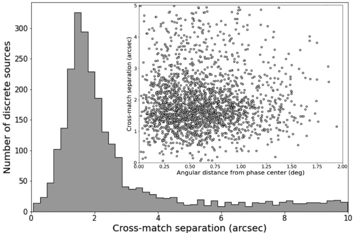
**Figure 1.** (top) Histogram of the cross-match separations between 2532 discrete compact sources from our MeerKAT FRB 20190714A field and *WISE* point source catalogue of the same field. The distribution of the histogram peaks at  $\sim 1''.5$ . (inset) A scatter plot of the angular distance from the phase center of the MeerKAT pointing against the cross-match separation up to 5 arcsec.
