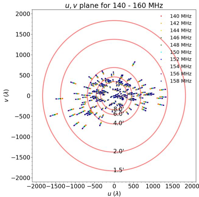
**Fig. 2.**  $u, v$  coverage for the multi-frequency band 140–160 MHz. Each of the coloured points on the  $u, v$  plane correspond to a different frequency observed for a given baseline. A series of red rings illustrate an example of the baselines which contribute to achieving a particular angular resolution for 140 MHz, i.e. the longer baselines are responsible for resolving the smaller structure.
